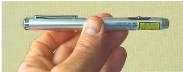
Inexpensive laser pointer (1 mW, 650 nm red).
