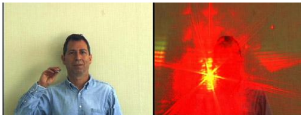
Laser pointer aimed at video camera from 3 meters away.
